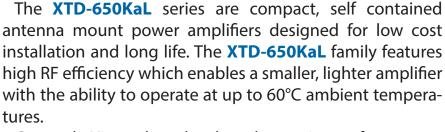
Comtech Xicom has developed proprietary features to improve performance and life including an automatic bias control system which extends TWT life by maintaining constant beam current over time and a precise system for matching linearizer performance to a specific tube over a wide range of operating conditions maximizing useable linear power.
